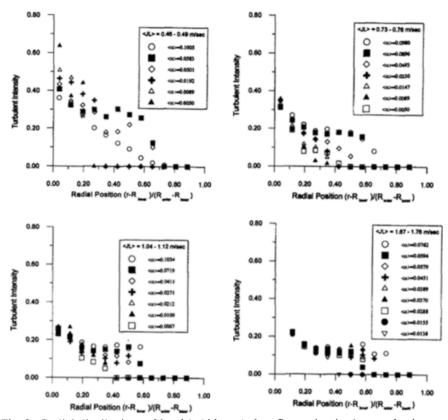
Fig. 8 Radial distributions of local bubble turbulent fluctuation in the annulus loop
