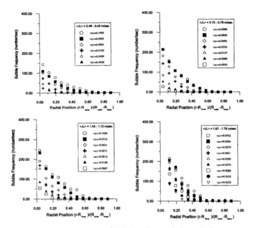
Fig. 4 Radial distributions of local bubble frequency in the annulus loop
